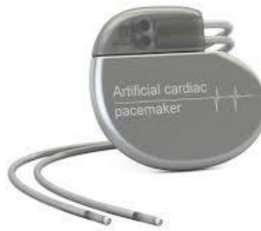
Figure 2. Pacemaker (Generator and Two Leads)
